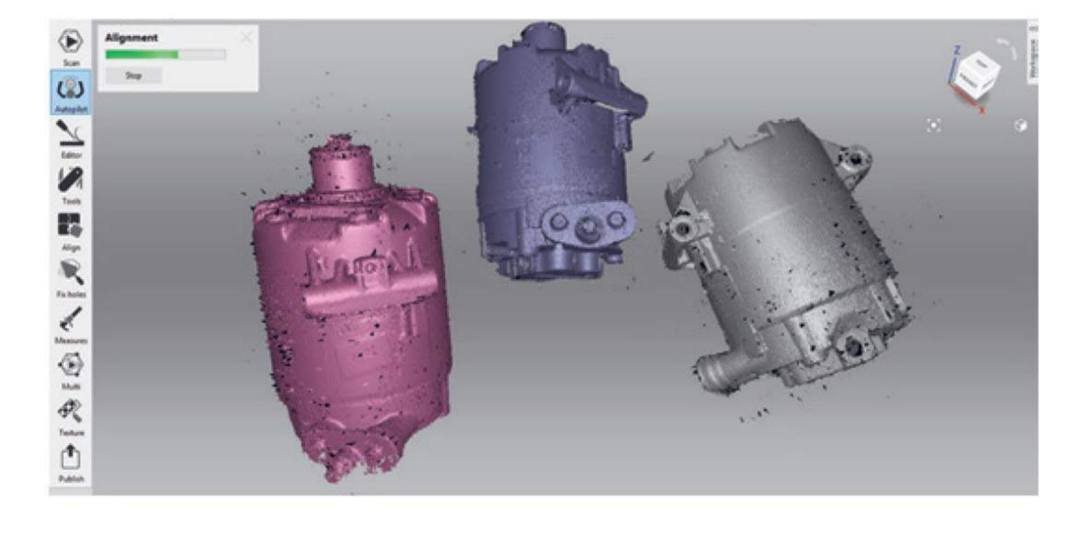
Step 3b Confirm that all scans are correctly aligned
